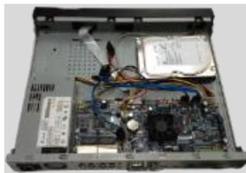
② Place the HDD in accordance with the four holes in the bottom.
