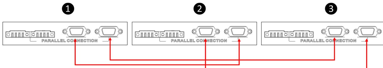
**WARNING:** Do NOT connect the current sharing cables between the inverters in different phases. Otherwise, it may damage the inverters.
