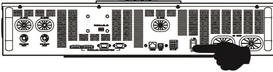
Once the unit has been properly installed and the batteries are connected well, simply press On/Off switch (located on the bottom of the inverter) to turn on the unit.
