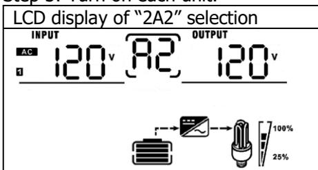
Step 4: Switch on all AC breakers of Line wires in AC input. It's better to connect all of the inverters to the utility at the same time. If not, it will display fault 82 in the following inverters. However, these inverters will automatically restart. If detecting AC connection, they will work normally.
