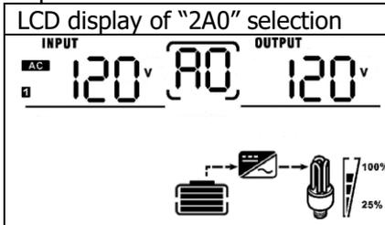
Step 4: Switch on all AC breakers of Line wires in AC input. It's better to connect all of the inverters to the utility at the same time. If not, it will display fault 82 in the following inverters. However, these inverters will automatically restart. If detecting AC connection, they will work normally.
