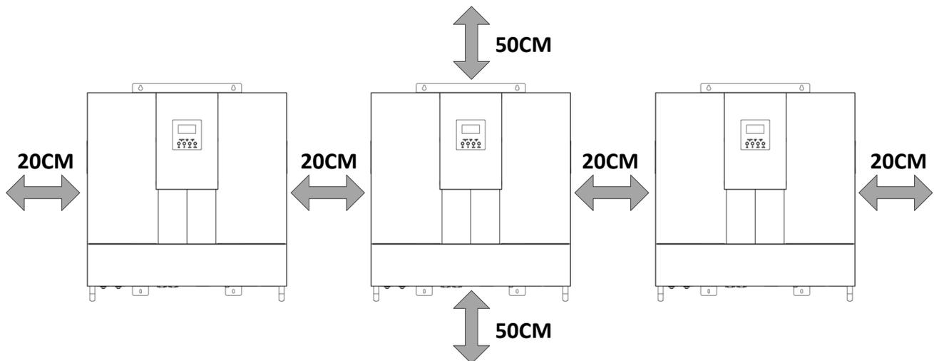
**NOTE:** For proper air circulation to dissipate heat, allow a clearance of approx. 20 cm to the side and approx. 50 cm above and below the unit. Be sure to install each unit in the same height.
